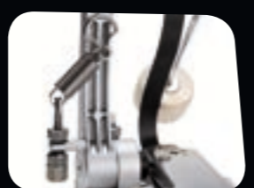
Spring hold by a magnet
